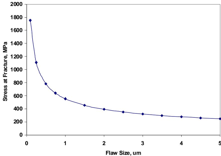
**Fig. 5:** The fracture toughness relationship between the length of a flaw (crack) and the maximum theoretical fracture strength of silicon in pure tension loading (Mode I). The fracture toughness,  $K_{IC}$ , of silicon is  $\sim 1.0 \text{ MPa}\cdot\text{m}^{1/2}$ .
