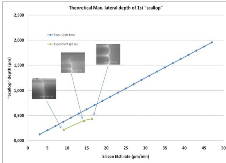
**Fig. 3** Scallop depth (sidewall roughness) versus silicon etch rate for a time-multiplexed silicon etch process.
