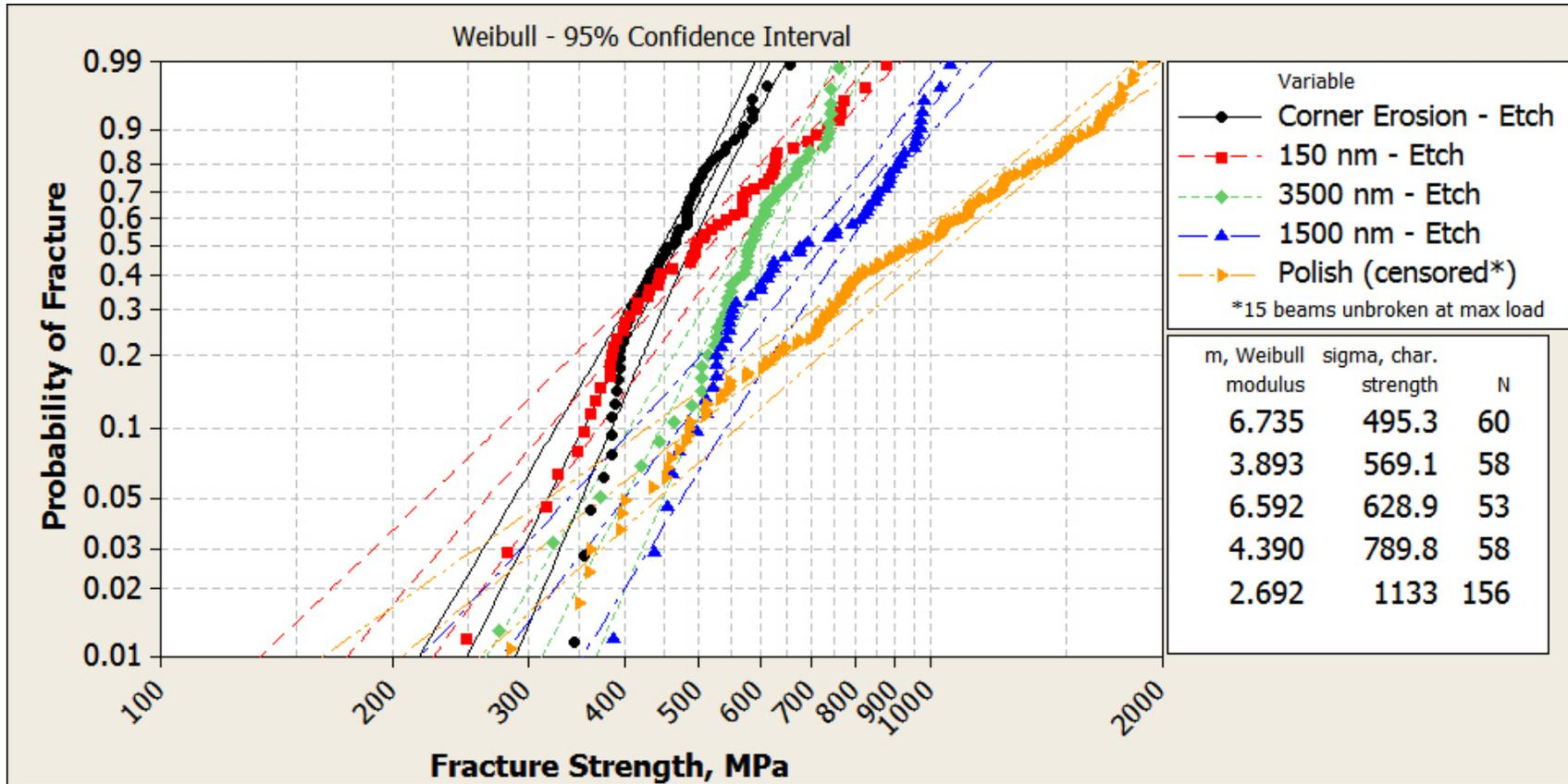
Fig. 8: Probability plot of the fracture test data from five different groups of specimens.
