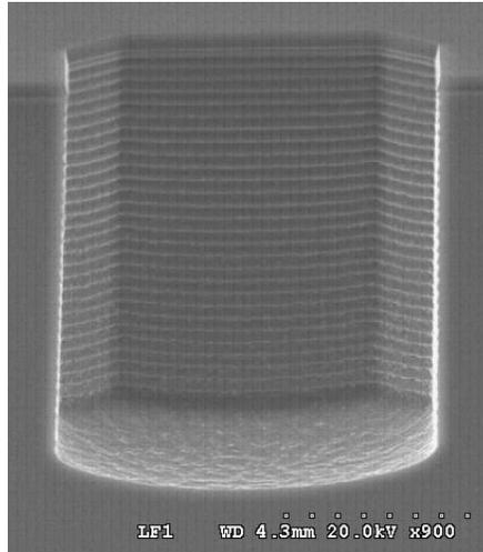
**Fig. 1** SEM micrograph of etched silicon feature showing characteristic Bosch process scallops.
