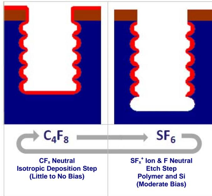
Fig. 2 Cyclical nature of Bosch process etching
