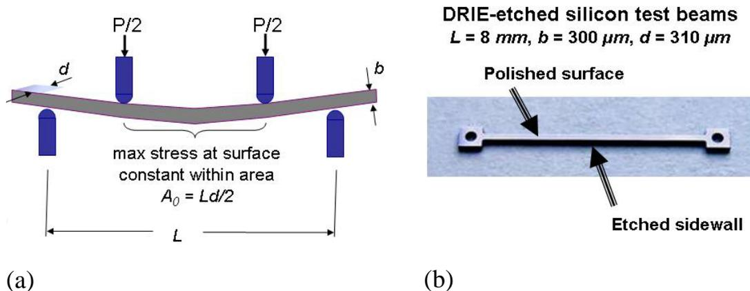
**Fig. 7:** (a) Diagram of the loading and geometry of a four-point bend specimen. (b) Photograph of a silicon test beam. The beam has four surfaces, two which have been etched, and two which are a standard polished wafer surface (semiconductor Prime grade).
